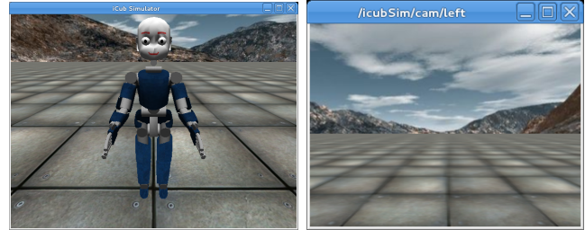
Fig. 1. An unmodified iCub simulator (left), streaming images directly to a ROS image_pipeline image_view instance (right). The images depart a TCP socket opened by the simulator in ROS sensor_msgs/Image format serialized to a TCPROS connection. No extra copy is made of the image, represented in the simulator in a non-ROS structure. The simulator source code is untouched by any of this, and no explicit bridging node is needed.
