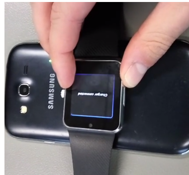
(d) Charging wirelessly a smartwatch with the smartphone
