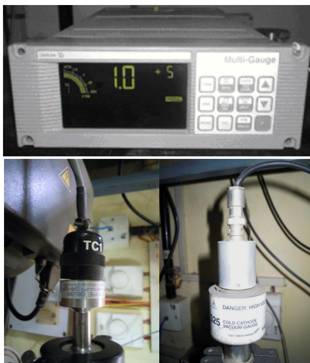
Figure 7. 16: multi pressure gauge controller, vacuum gauge and 525 Cold Cathode Ionization Gauge Tube.
