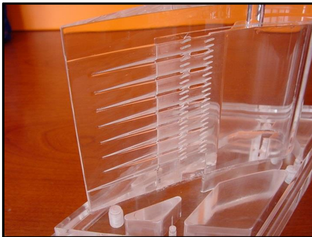
Figure 2.5 : Plexiglas ® blade and internal cooling system .
