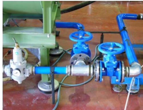
Fig. 3.24- Pipes connection between the compressor manifold and the plenums ( up ); Regulating valves ( down right ), Electrical heaters placed inside the pipe ( down left )
