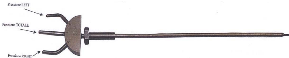
Fig. 3.12- The 3-hole probe (wedge type) used in this study
