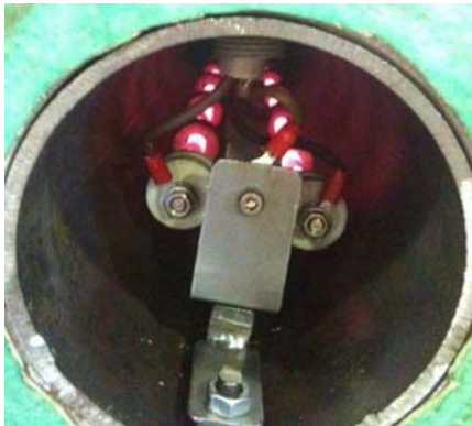
Fig. 3.24- Pipes connection between the compressor manifold and the plenums ( up ); Regulating valves ( down right ), Electrical heaters placed inside the pipe ( down left )
