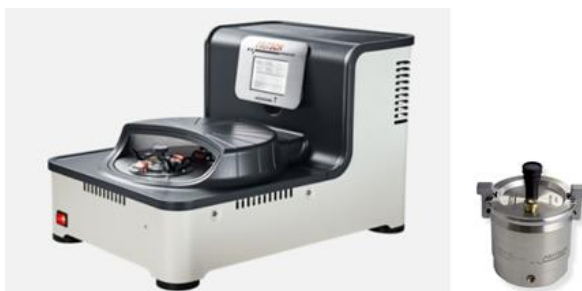
Figure 3.11 Fitsch Pulverisette 7 Premium Line and zirconium oxide grinding bowl with stainless casing
