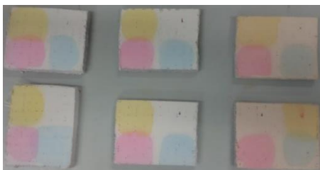
Figure 3.1 Preliminary studies to choose the model dye to determine the self-cleaning performances of the paint.
