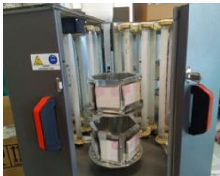
Figure 5.5 Photoreactor (Multirays) and ad-hoc prepared support with the specimens
