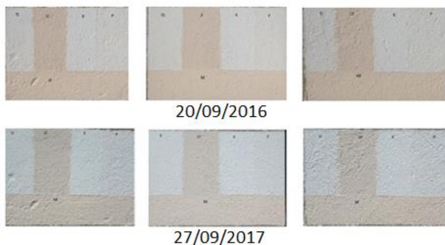
Figure 5.13: Photographs of the three small areas coated with the five types of paint (Ti, LF, K, P and M). The top three correspond to the initial moment and the bottom three portray the areas after one year of nature exposure.
