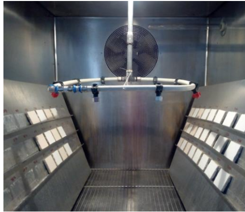
Figure 5.3 Weathering chamber with samples before starting the last 20 cycles.
