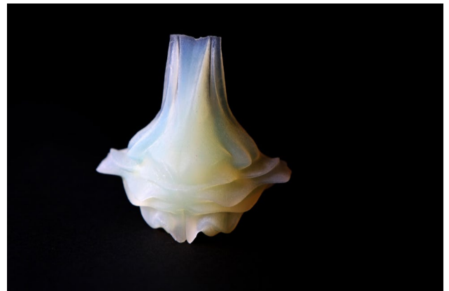
Figure 8 | Nose project Radiator / resonator – photo of 3D printed object in Flexible material Tango Plus 9740. Technology polyjet, solidified liquid photopolymer by using UV light (front view).
