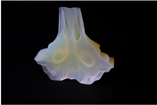
Figure 9 | Nose project Radiator / Resonator – photo of 3D printed object in Flexible material Tango Plus 9740. Technology polyjet, solidified liquid photopolymer by using UV light (back view).
