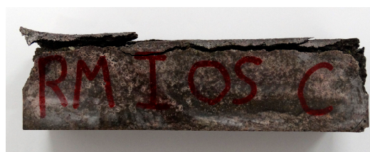
Figure 18. Specimen manufactured with CEM I 42.5R after 14 days in 30 wt % \text{CaCl}_2 solution at 4 °C.
