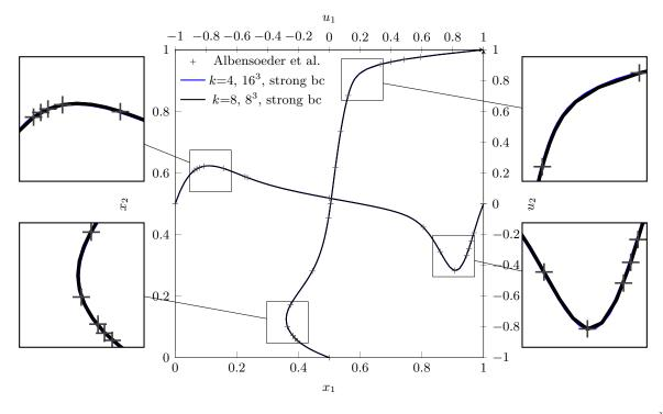
Figure 8: 3D Lid-driven cavity flow, horizontal component  $u_1$  of the velocity along the vertical centerline  $x_1, x_3 = \frac{1}{2}$  and the vertical component  $u_2$  of the velocity along the horizontal centerline  $x_2, x_3 = \frac{1}{2}$  for Re = 1,000
