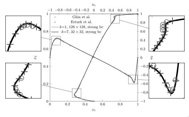
Figure 4: 2D Lid-driven cavity flow, horizontal component  $u_1$  of the velocity along the vertical centerline  $x_1 = \frac{1}{2}$  and the vertical component  $u_2$  of the velocity along the horizontal centerline  $x_2 = \frac{1}{2}$  for Re = 5,000
