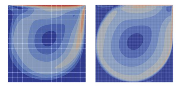
Figure 1: Two-dimensional lid-driven cavity flow, velocity magnitude contours (10 equispaced values in the range [0,1]) for k=7 computations at Re = 1,000 (left: 16x16 grid) and Re = 20,000 (right: 128x128 grid).
