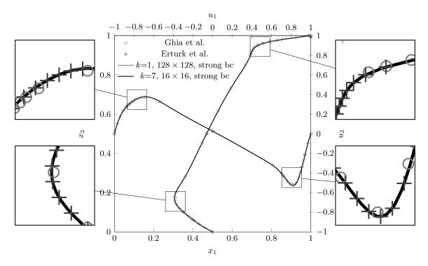
Figure 3: 2D Lid-driven cavity flow, horizontal component  $u_1$  of the velocity along the vertical centerline  $x_1 = \frac{1}{2}$  and the vertical component  $u_2$  of the velocity along the horizontal centerline  $x_2 = \frac{1}{2}$  for Re = 1,000
