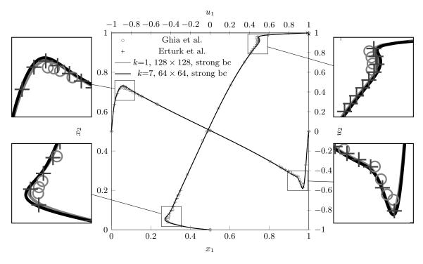
Figure 5: 2D Lid-driven cavity flow, horizontal component  $u_1$  of the velocity along the vertical centerline  $x_1 = \frac{1}{2}$  and the vertical component  $u_2$  of the velocity along the horizontal centerline  $x_2 = \frac{1}{2}$  for Re = 10,000
