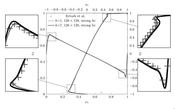
Figure 6: 2D Lid-driven cavity flow, horizontal component  $u_1$  of the velocity along the vertical centerline  $x_1 = \frac{1}{2}$  and the vertical component  $u_2$  of the velocity along the horizontal centerline  $x_2 = \frac{1}{2}$  for Re = 20,000
