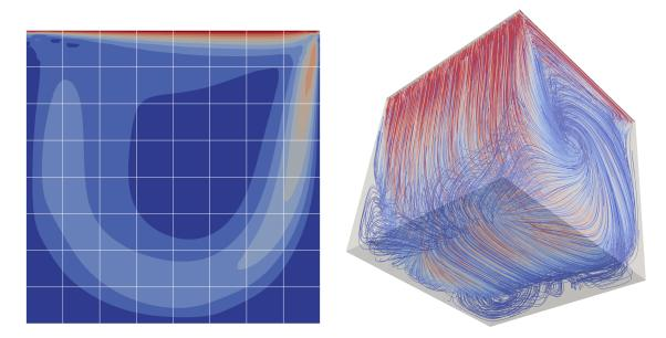
Figure 2: Three-dimensional lid-driven cavity flow at Re = 1,000 computed by means of a k=8,  $8^3$  hexahedral elements grid HHO discretization. Left, velocity magnitude contours (10 equispaced values in the range [0,1]) over the vertical mid-plane whose top edge is aligned with the velocity vector. Right: Streamlines color-coded by velocity magnitude.
