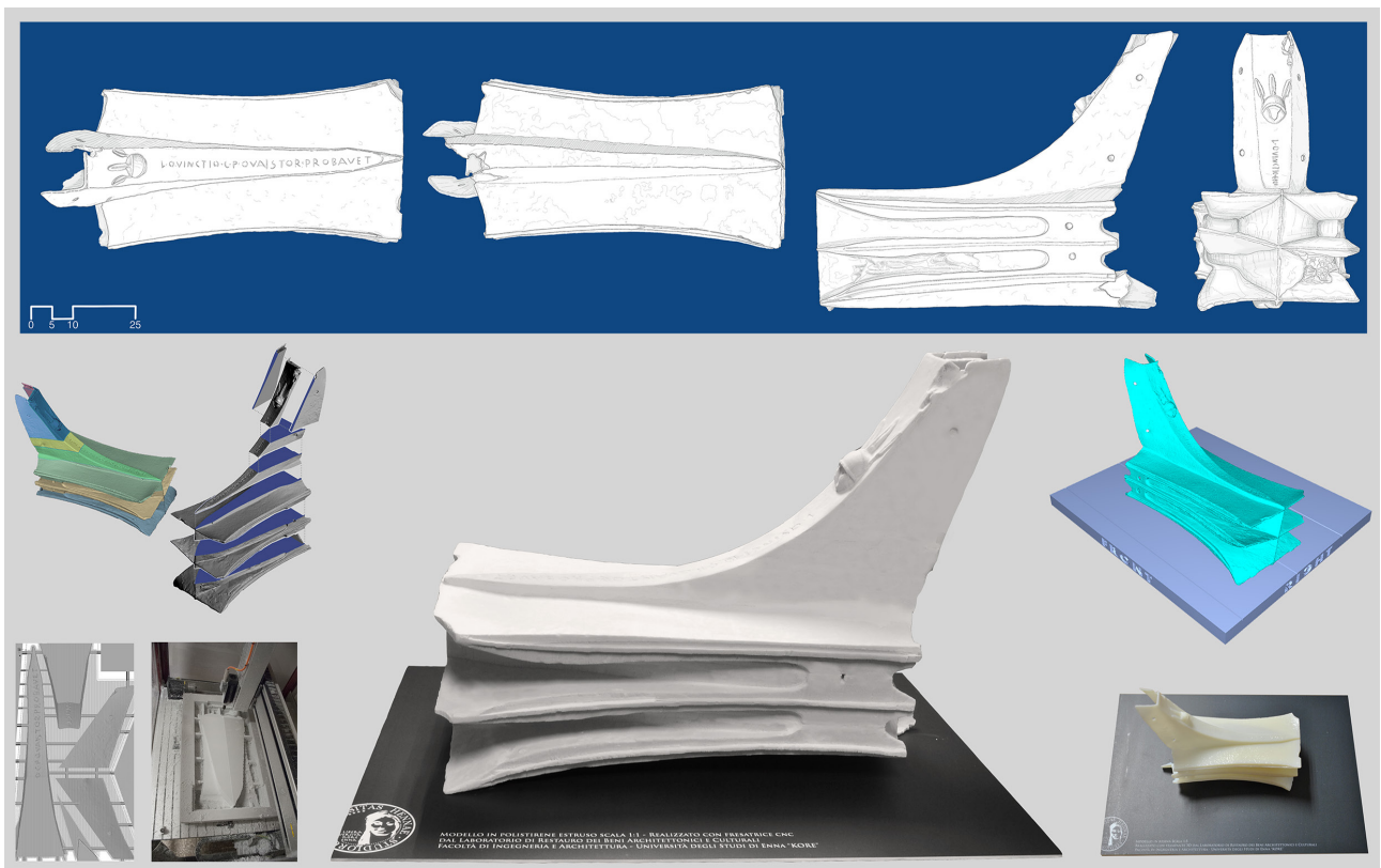
Figure 7. Maquette of the rostrum realised in scale 1: 1 by CNC machine.
