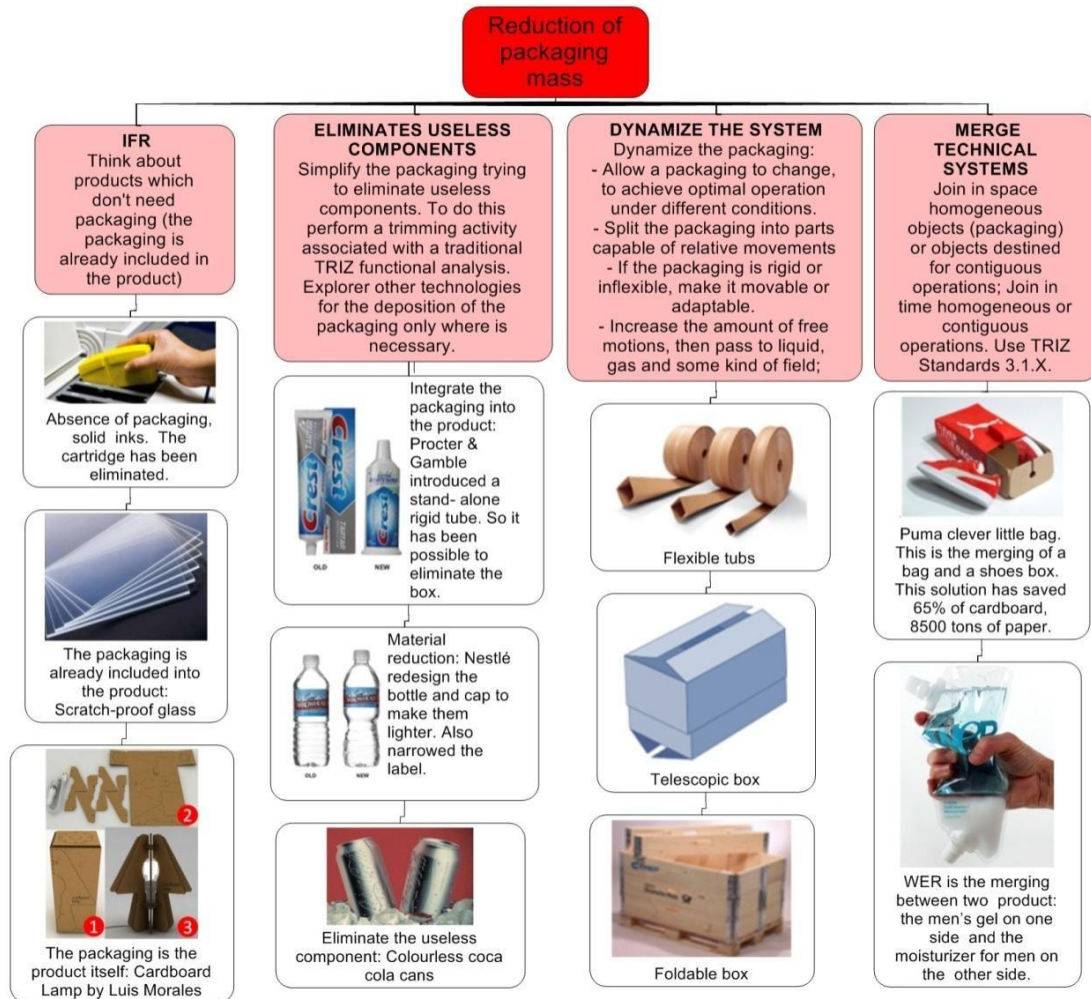
Figure 6. Example of a set of the 330 guidelines dealing with how to “reduce the packaging mass”.
