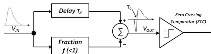
**Figure 5.** Scheme of CFD principle of operation.
