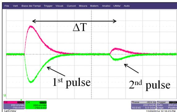
**Figure 10.** Input signals for double pulse test.
