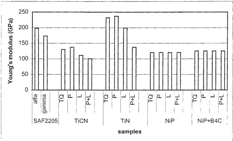
Figure 5: Young's modulus of bulk and thin film plated on different finishing surface conditions
