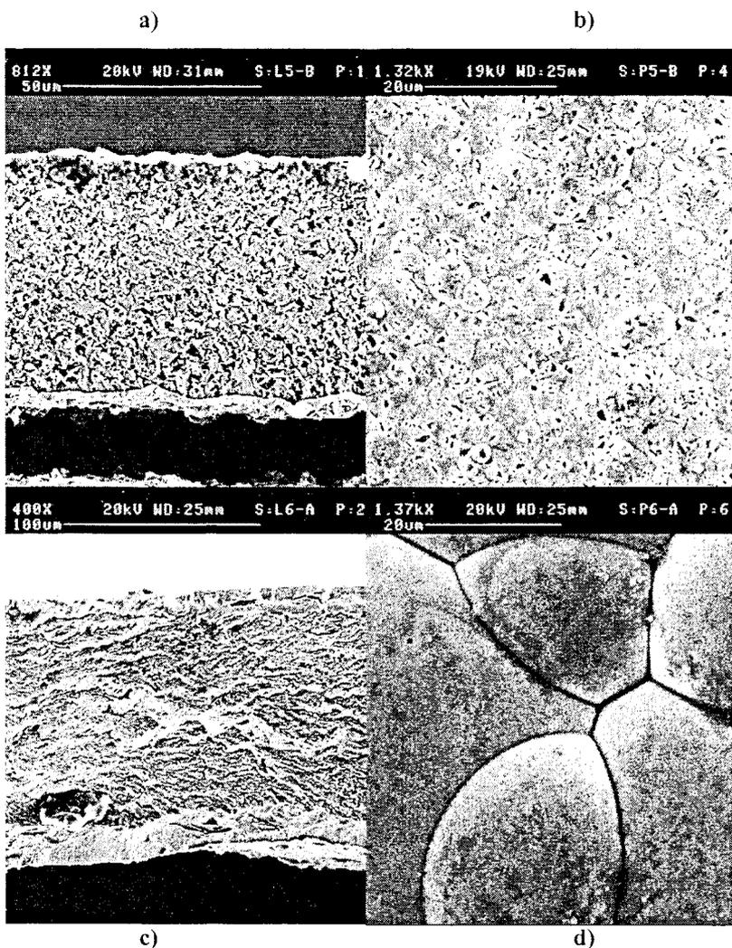
Figure 4: Ni-B<sub>4</sub>C coating: a) cross section, b) surface morphology; Ni-P coating: c) cross section, and d) surface morphology.
