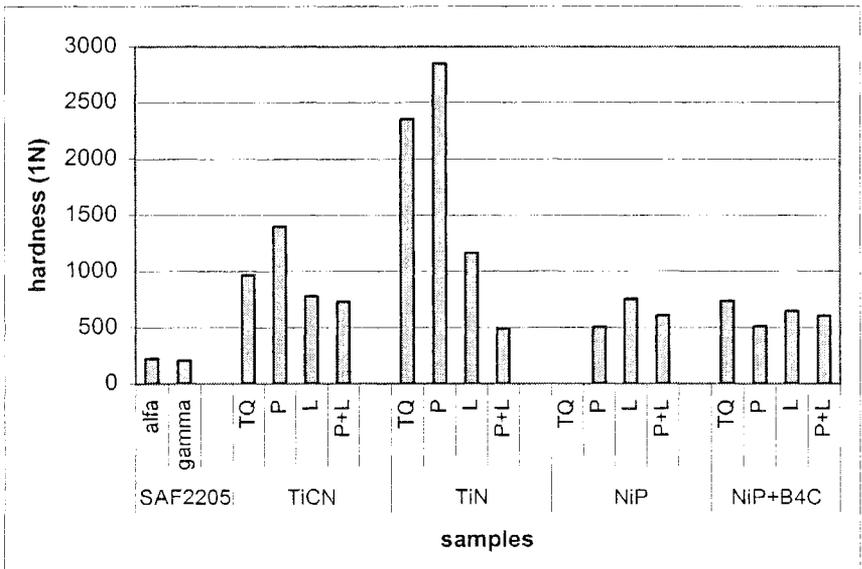
Figure 1: microhardness measurement of bulk and thin films plated on different finishing surface conditions
