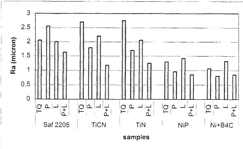
Figure 2: roughness measurement of bulk and thin film plated on different finishing surface conditions
