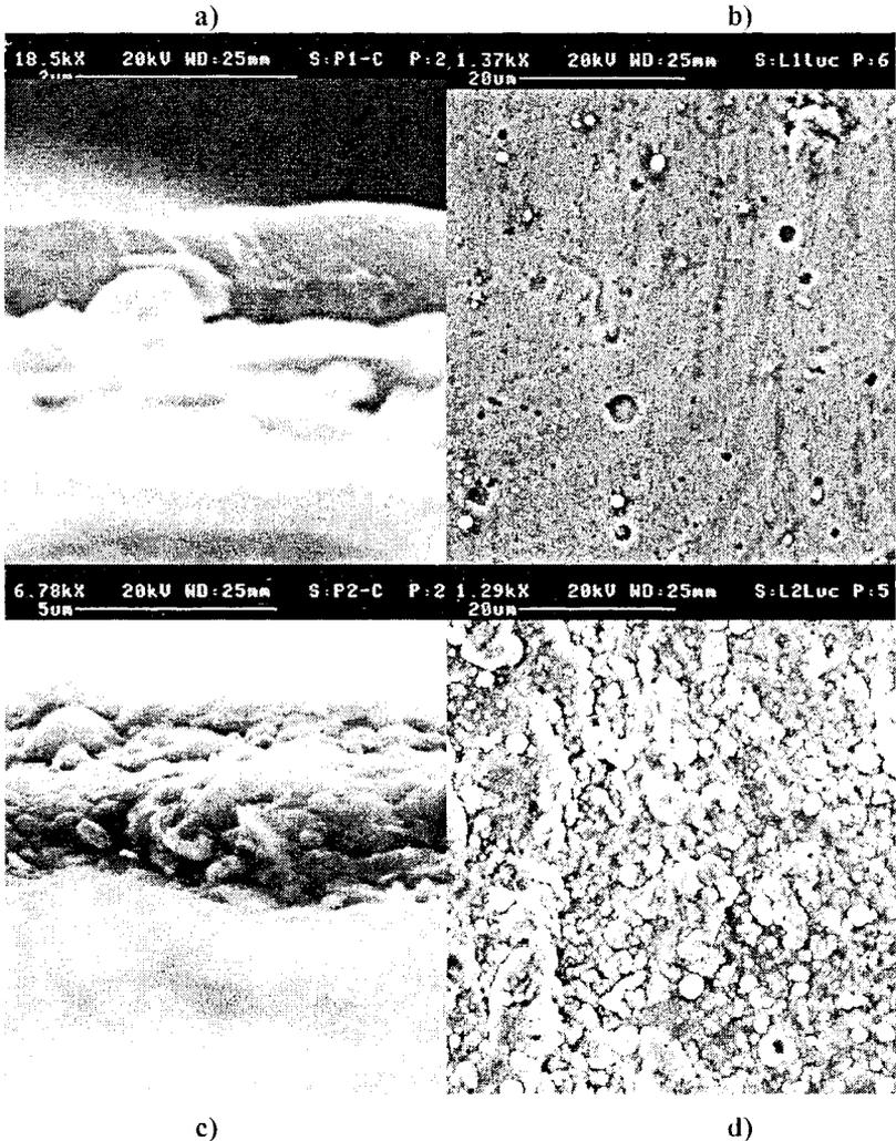
Figure 3: TiN coating: a) cross section, b) surface morphology; TiCN coating: c) cross section, and d) surface morphology.
