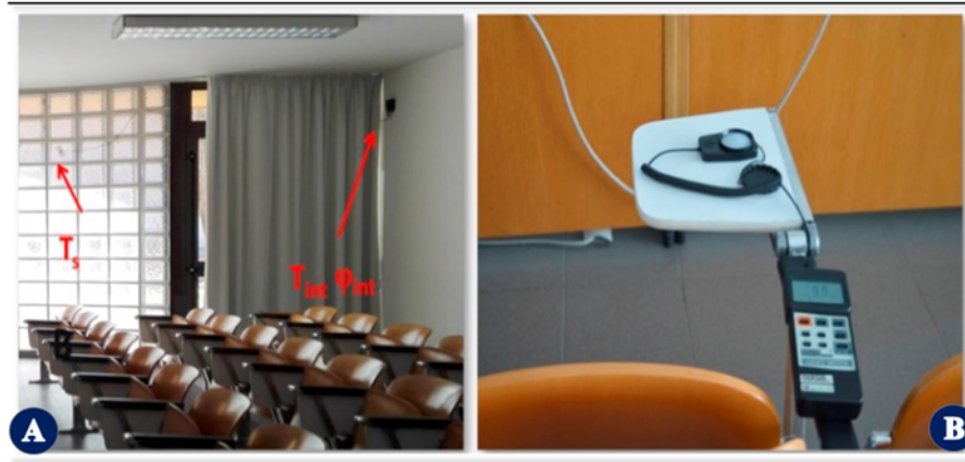
Figure 93: classroom 5: (a) sensors for temperatures and relative humidity; (b) light level measure.
