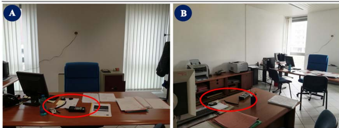
Figure 100: Installed sensor for light level measure: (a) desk1 and (b) dek2.
