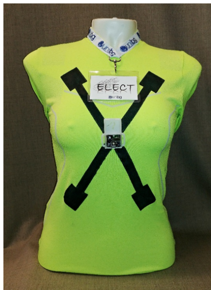
Fig. 3.15. “ELECT”, smart textile for the heart rate monitoring through ECG.
