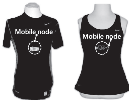
Figure 2.64 – Photograph of the ECG device mounted on male and female shirts presented by Lee et. al.
