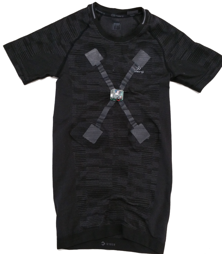
Figure 2.60 – Prototype of the t-shirt with conductive traces.
