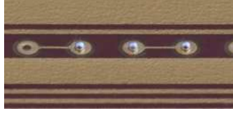
Figure 4.18: A detail of the prototype sample for laser soldering test: three solder balls of 250\text{ }\mu\text{m} diameter placed on top of the chip and FPC prior to laser soldering are visible
