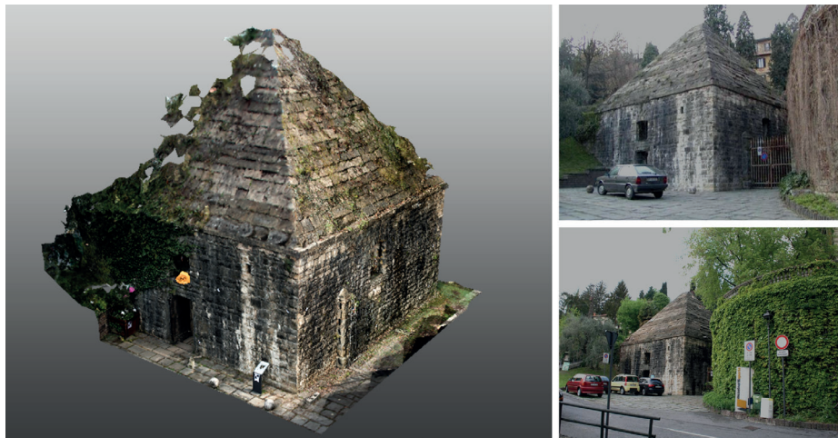
Fig. 2. The 'Torresino da Polvere' in via Beltrami in Bergamo; on the left the preview of the 3D model (projection of the photogrammetric model on the 3D laser scanner point cloud); on the right of the photographic images of the architecture after the restoration work of the years 1980.
