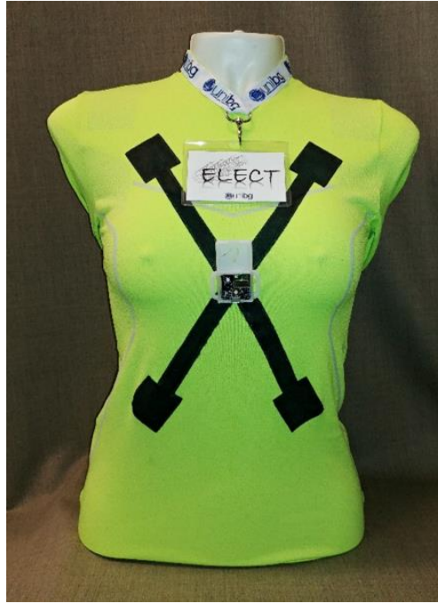
Figure 15: “ELECT”, smart textile for the heart rate monitoring through ECG
