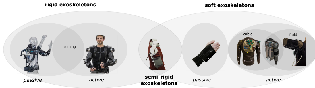
Figure 1.1: Classification of the wearable robots in: (i) rigid exoskeletons; (ii) semi-rigid exoskeletons; (iii) soft exoskeletons.
