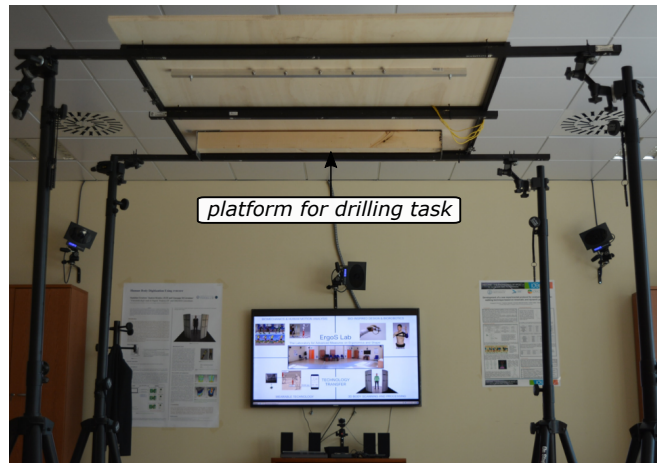
Figure 2.2: Front view of the experimental setup comprising four poles as based and overhead platform to perform drilling, leveraging and cabling tasks.
