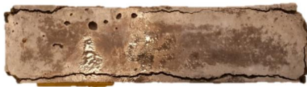
Figure 3-17 PC specimen after 42 days in \text{CaCl}_2 -rich solution
