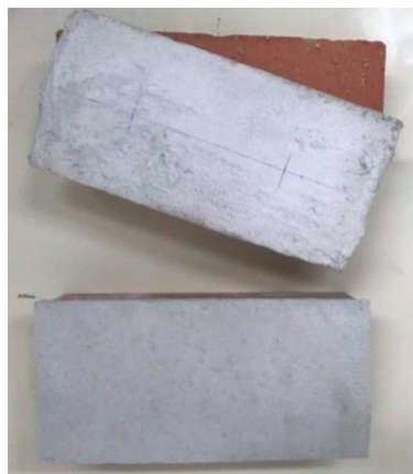
Figure 4-4 Test on a brick: S8 4:1 detached and S8 4:1_def adherent
