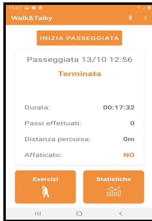
Figure 1. A screenshot of the Walk&Talky application, developed by MediaClinics. The screen shows the data of a performed walk, i.e., walk duration, steps, walked distance, detected fatigue state. Plus, there are two buttons in the lower part of the screen that allow participants to, respectively, access a library of exercises to be done at home and access the statistics on all the performed walks.
