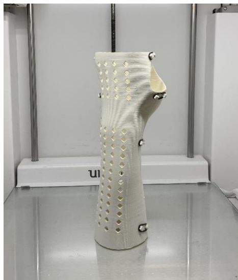
Figure 56. Prototype of wrist immobilisation splint made in PLA with a 3 mm surface thickness.
