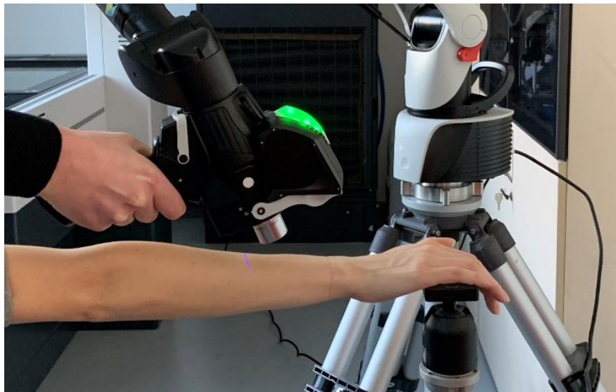
Figure 45. Optimal configuration of the 3D limb geometry acquisition with the Hexagon Absolute Arm 7-Axis equipped with RS6 Laser Scanner.
