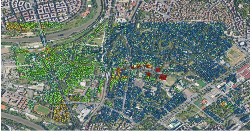
Figure 13: Representation of deformation velocities for an urban area in Rome (QGIS).
