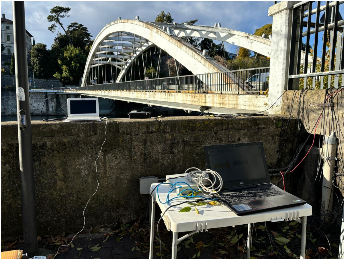
Figure 99: Experimental setup for dynamic data acquisition.
