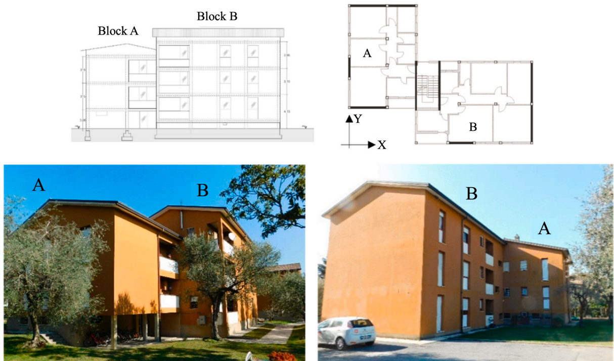
Fig. 3. Blocks A and B elevation and plan (top), and prospects (bottom) (adapted from Ref. [1]).
