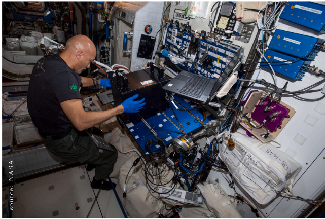
Fig. 3. Luca Parmitano prepares the Multiscale Boiling EC for installation within the FSL.
