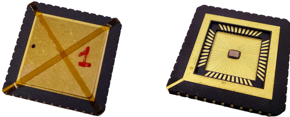
(a) External view of the CLCC44 package of the antares4_001 ASIC with the lid closed, showing the protective metal lid and package enclosure. (b) Internal view of the same package with the lid removed, revealing the ASIC die glued to the cavity and connected to the pads through wire bonds.
