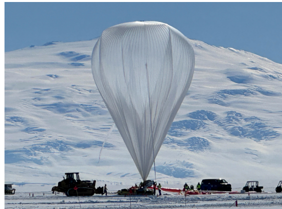
(b) Inflation of the scientific balloon at the NASA LDB launch site prior to the first GAPS flight campaign.
