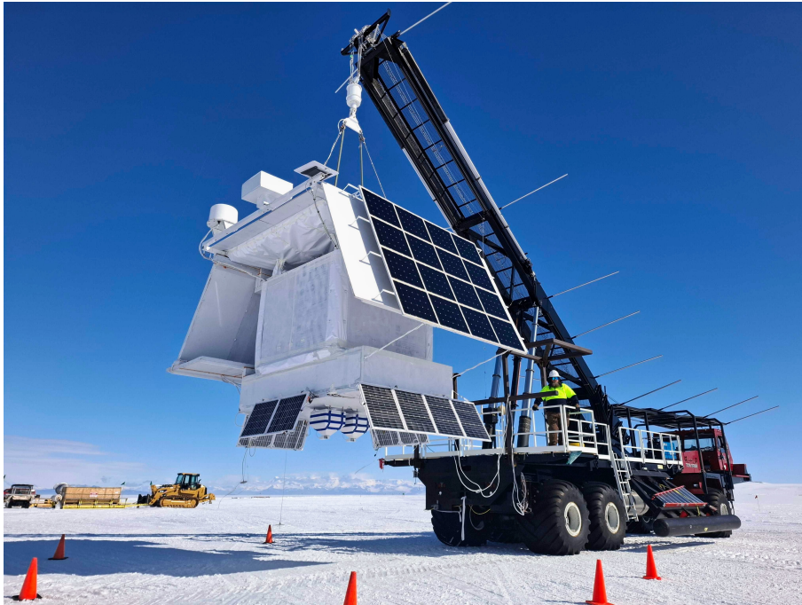
Figure 1.6 The GAPS instrument in its flight-ready configuration, suspended from the launch vehicle at the NASA Long Duration Balloon (LDB) facility at McMurdo Station, Antarctica. Picture courtesy of Philip von Doetinchem.
