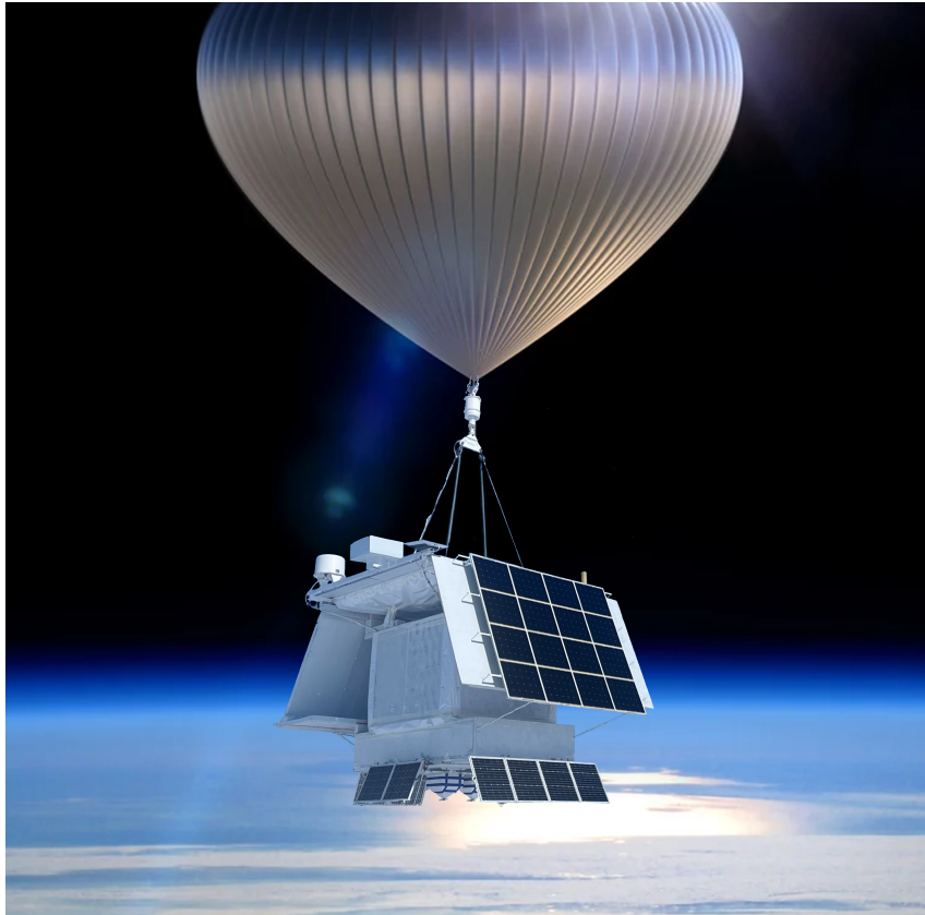
Figure 1.7 Rendering of the GAPS instrument in flight, suspended from a high-altitude scientific balloon during Antarctic operations. The balloon is not to scale with respect to the instrument. The image illustrates the instrument’s configuration at float altitude. Picture courtesy of Kelsey Lee.
