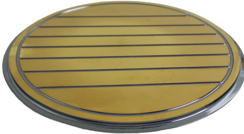
Figure 2.4 Photograph of a fabricated eight-strip GAPS Si(Li) detector. The image shows the top ( n -side) surface with etched grooves that electrically isolate the strips and define the outer guard ring. These circular detectors have a diameter of 10 cm and a typical thickness of \sim 2.5 mm, optimized to provide sufficient stopping power for low-energy cosmic-ray antiparticles while allowing efficient escape and detection of de-excitation x-rays. Picture courtesy of the GAPS collaboration.
