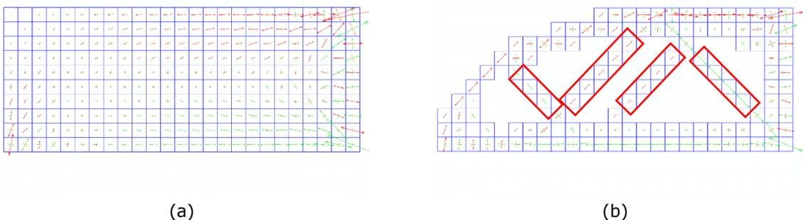
**Figure 2:** Stress fields for original and optimized structure. The analysis has been carried out using Abaqus while the optimization implementing the BESO algorithm.
