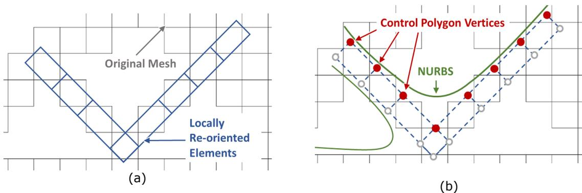
**Figure 6:** NURBS application: (a) re-oriented elements, (b) definition of fitting NURBS.
