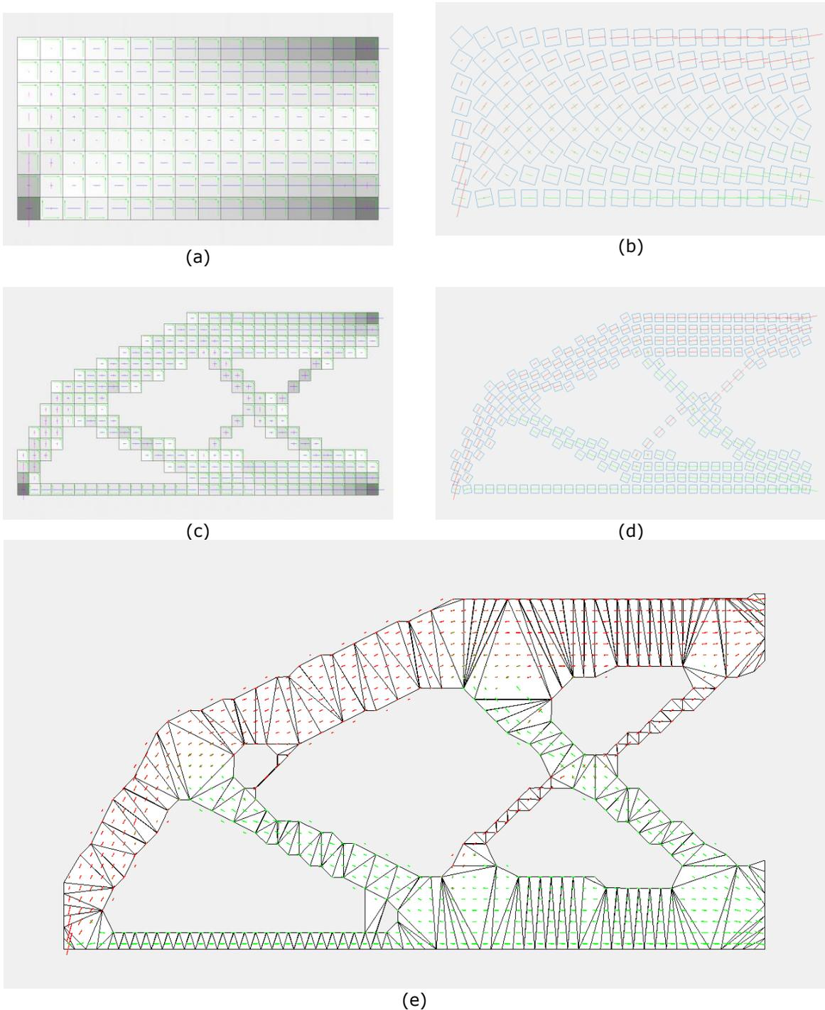
**Figure 4:** MATLAB implementation: (a) and (d) are the results of the FEA on the design space; (c) and (d) depict the FEA analysis carried out on the result of the BESO TO procedure; (e) shows the result of the proposed approach.
