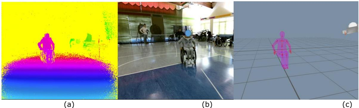
**Figure 1:** Depth data (a) and RGB data (b) acquired with Kinect devices through iPi Recorder and the virtual avatar computed by iPi Mocap Studio (c).
