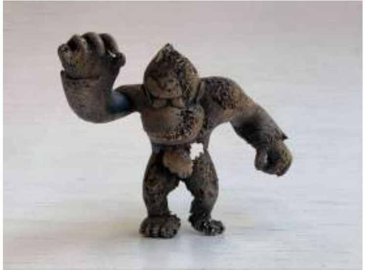
Fig. 2. The hole in the side of this sculpture was caused by an air pocket, whereas the texture on its surface was caused by the metal hardening before it could fill in the entire. A patina was then applied to darken and highlight these textures, using them as sculptural features left by the process. Image by Elizabeth Tsu (2021).
