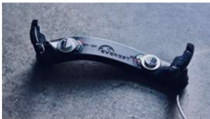
Fig. 1. The vibrotactile shoulder rest I use with my augmented violin.
