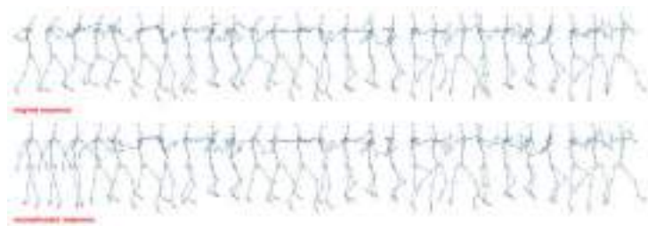
Fig. 3. Pose Sequence Reconstruction Test. The figure depicts the first 30 seconds of an original (top) and reconstructed (bottom) pose sequence with individual poses drawn at ten frames intervals. The deviation between the two sequences at their beginning is due to the SLERP algorithm gradually fading in a pose sequence on top of a base pose with which the result pose sequence has initially been populated with.
