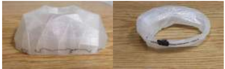
Fig. 6. The plastic original of a 3D printed object to be sand cast. Markings in black clay and pen are modifications suggested by the foundry operator. These changes to the geometry of the object were trivial to make to the original CAD files, meaning a new object could be printed the same day. Image by author.
