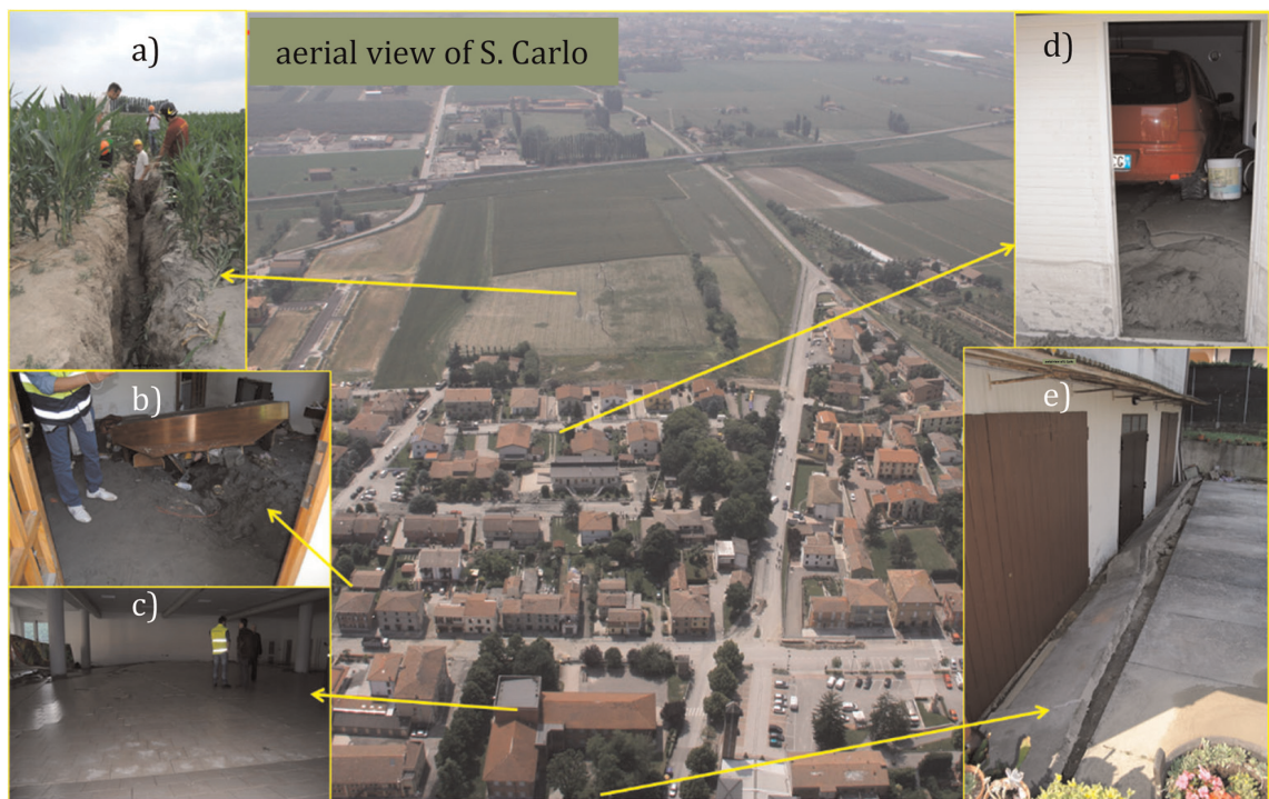
Figure 1. Evidence of liquefaction registered in Italy in 2012 at the site of S. Carlo: (a) external inhabited areas, extensional crack due to lateral spreading; (b) ground floor flooded by erupted sand; (c) basement floor lifted by sand under pressure; (d) car lifted up by the ejected sand; (e) building settlement.
