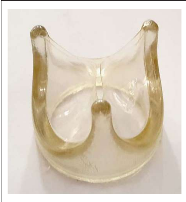
Figure 1. Final dip-casted 25-mm polyurethane valve.
