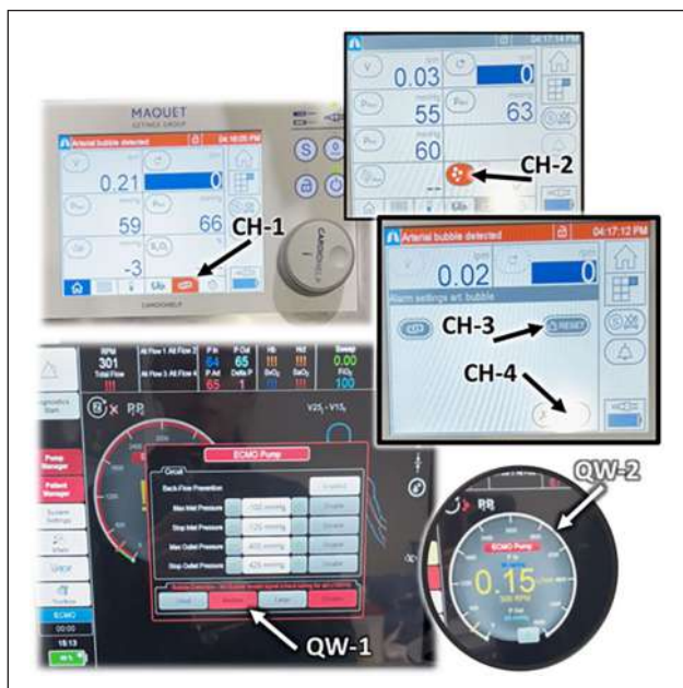
Figure 1. The touches and menu navigation required to resume pump speed after an ABD alarm for the CardioHelp (CH) and Quantum Workstation (QW).
