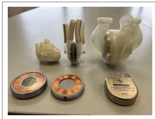
Figure 1. Size comparison Top from left: 5 years old heart model, resulted artificial heart, Bivacor TAH model; Bottom: Subcutaneous driver, smart battery, Medtronic Protecta XT CRT
