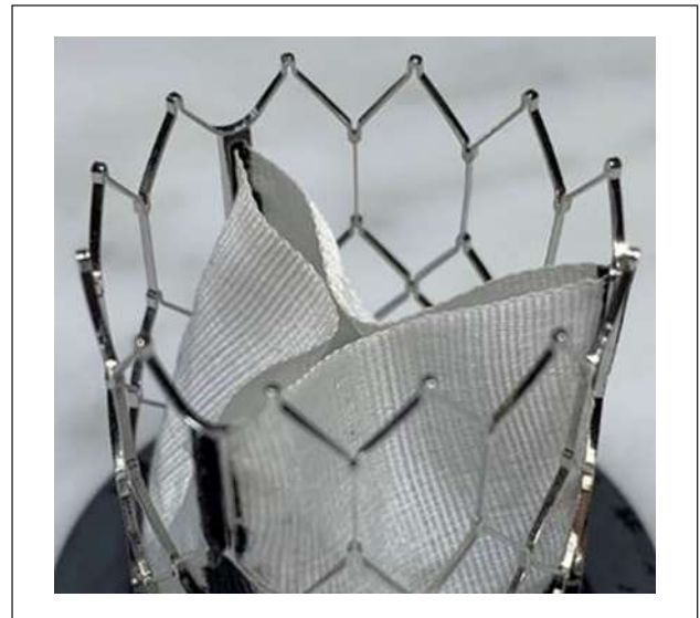
Figure 1. Textile heart valve scaffold tested with 200 million load cycles.
