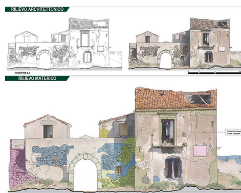
Fig. 4 – Orthophotos and 2D drawings for materials' mapping.
