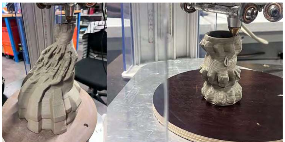
Fig. 17. Streamline pieces being 3D-printed.
