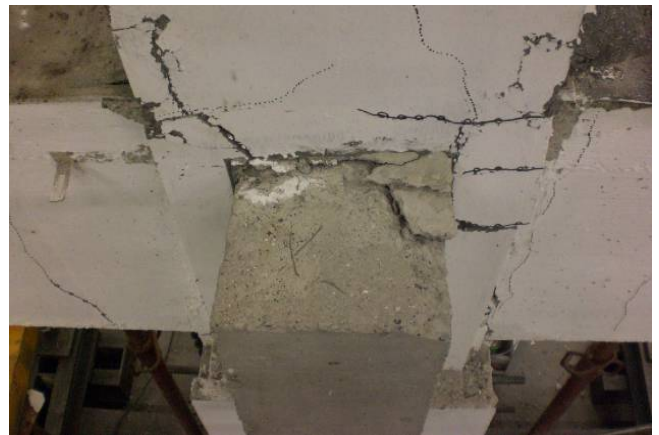
Figure 12. Cracks in the region with corbel interface.
