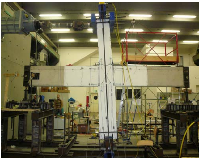
Figure 10. Specimen at a drift equal to \pm 4\% .
